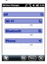
The status fields below the Wi-Fi button, the Bluetooth button, and the Phone button change from Off when the radios are turned on and show the current state of the radio. The Wi-Fi status field shows Connecting or Available, the Bluetooth status field shows *On* or *Visible*, and the **Phone** status field shows *On* or the name of the cellular network that you are connected to.
