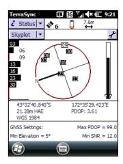
are too weak. In the example shown here, eight satellites are being tracked and seven of these satellites are being used to compute GPS positions.
